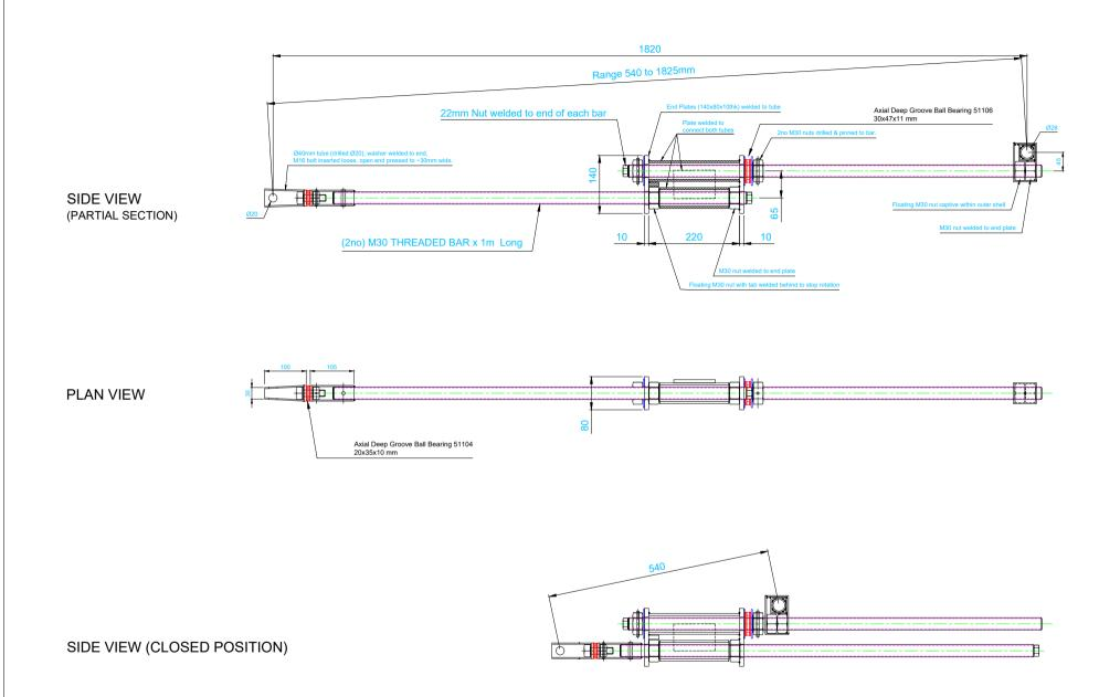
SBU CAB LIFT MECHANISM
